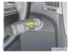
If the battery is weak or the smart key does not work correctly, you can start the engine by pressing the engine start/stop button with the smart key.
