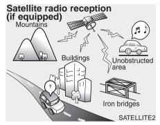
Satellite radio reception requires direct line of sight with the satellite transmitting the radio signal.
