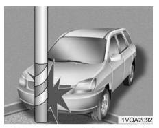
Air bags may not inflate if the vehicle collides with objects such as utility poles or trees, where the point of impact is concentrated to one area and the full force of the impact is not delivered to the sensors. C041100AUN
