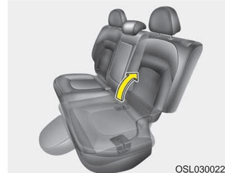
5. When you return the seatback to its upright position, always be sure it has locked into position by pushing on the top of the seatback.
