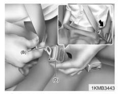
3.Pull the webbing and insert the tongue plate (B) into the open end of the buckle (D) until an audible "click" is heard, indicating the latch is locked. Make sure the belt is not twisted.
