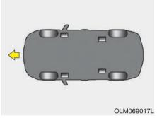
Tie-down hook (for flatbed towing, if equipped)
