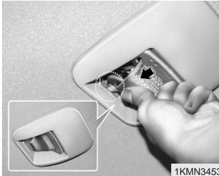
3. Insert the tongue plate into the hole on the belt assembly cover.
