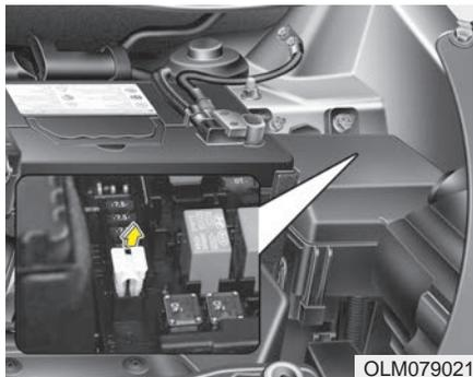
3. Pull the suspected fuse straight out. Use the removal tool provided on the engine compartment fuse panel cover.
