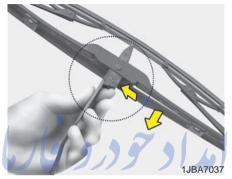
2.Compress the clip and slide the blade assembly downward.
