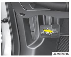
Releasing the parking brake Foot type
