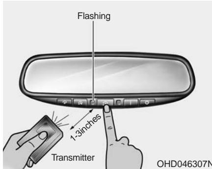
2. Press and hold the button on the HomeLink® system you wish to train and the button on the transmitter while the transmitter is approximately 2-8 cm (1 to 3 inches) away from the mirror. Do not release the buttons until step 3 has been completed.
