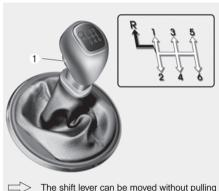
The shift lever can be moved without pulling the R knob (1).
