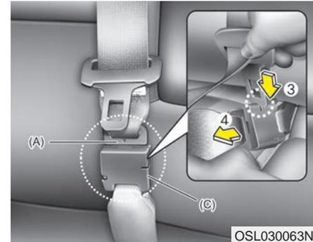
2. To retract the rear center seatbelt, insert the tongue plate or similar small rigid device into the webbing release hole (C). Pull up on the seat belt webbing (A) and allow the webbing to retract automatically.
