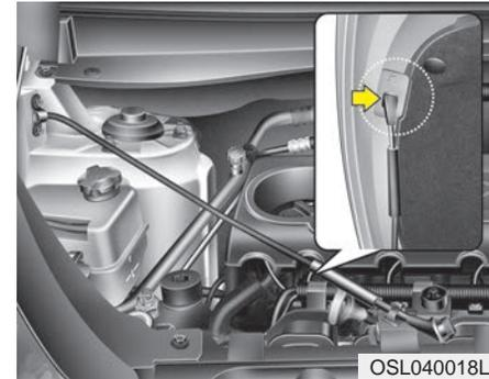
3. Pull out the support rod from the support rod holder.
