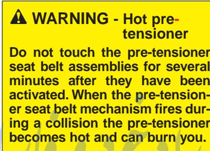
Pre-tensioners are designed to operate only one time. After activation, pre-tensioner seat belts must be replaced. If the pre-tensioner must be replaced, contact an authorized Kia dealer.
