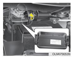
Engine compartment fuse panel
