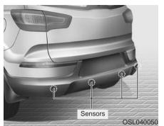
The Back up warning system assists the driver during backward movement of the vehicle by chiming if any object is sensed within a distance of 120 cm (47 in.) behind the vehicle.
