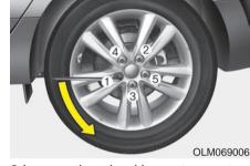
6.Loosen the wheel lug nuts counterclockwise one turn each, but do not remove any nut until the tire has been raised off the ground.
