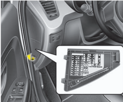
Inner fuse panel
