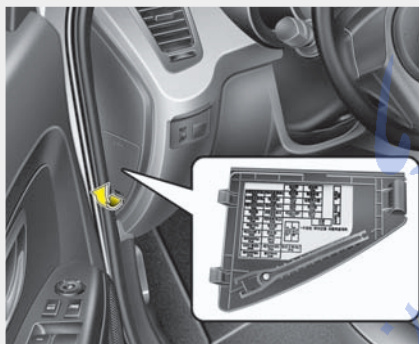
Inner fuse panel
