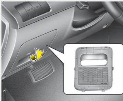
Inner fuse panel
