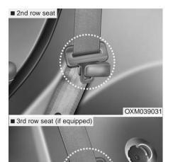
Routing the seat belt webbing through the rear seat belt guides will help keep the belts from being trapped behind or under the seats.
