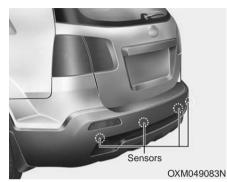
The rear parking assist system assists the driver during backward movement of the vehicle by chiming if any object is sensed within a distance of 47 in. (120 cm) behind the vehicle.
