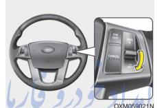
Push the - SET switch, and release it at the desired speed. The SET indicator light in the instrument cluster will illuminate. Release the accelerator at the same time. The desired speed will automatically be maintained.
