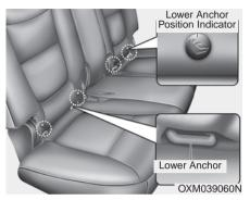
Child restraint symbols are located on the left and right 2nd row seat backs to indicate the position of the lower anchors for child restraints
