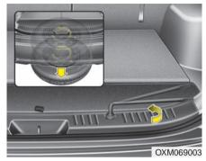
Use the wheel lug nut wrench to loosen the bolt enough to lower the spare tire.
