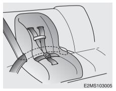
Installing a child restraint system with a lap/shoulder belt
