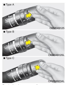
Push the lever away from you to spray rear washer fluid and to run the rear wipers 1~3 cycles. The spray and wiper operation will continue until you release the lever.
