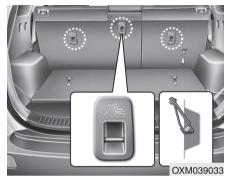
Securing a child restraint seat with tether anchor system (if equipped)
