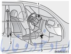
The seat belt pre-tensioner system consists mainly of the following components. Their locations are shown in the illustration: \_ \ \ \ > تلفن شبانه روزي. 1. SRS air bag warning light
