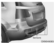
The rear parking assist system assists the driver during backward movement of the vehicle by chiming if any object is sensed within a distance of 120 cm (47 in.) behind the vehicle.
