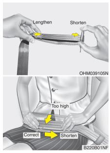
With a 2-point static type seat belt, the length must be adjusted manually so it fits snugly around your body. Fasten the belt and pull on the loose end to tighten. The belt should be placed as low as possible on your hips, not on your waist. If the belt is too high, it could increase the possibility of injury in an accident.
