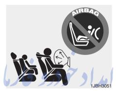
Do not install a child restraint on the front passenger's seat.
