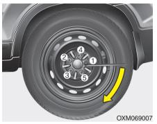
Then position the wrench as shown in the drawing and tighten the wheel nuts. Be sure the socket is seated completely over the nut. Do not stand on the wrench handle or use an extension pipe over the wrench handle. Go around the wheel tightening every other nut until they are all tight. Then double-check each nut for tightness. After changing wheels, have an authorized KIA dealer tighten the wheel nuts to their proper torque as soon as possible.
