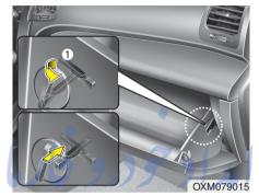
1. Open the glove box and remove the support strap (1).
