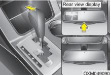
The rearview camera will activate when the back-up light is ON with the ignition switch ON and the shift lever in the R (Reverse) position.
