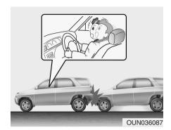
Air bags are not designed to inflate in rear collisions, because occupants are moved backward by the force of the impact. In this case, inflated air bags would not be able to provide any additional benefit.
