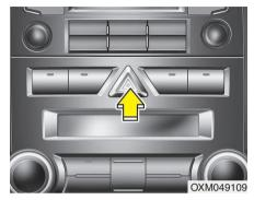
The hazard warning flasher should be used whenever you find it necessary to stop the vehicle in a hazardous location. When you must make such an emergency stop, always pull off the road as far as possible.
