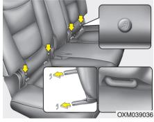
Both rear outboard seats are equipped with a pair of ISOFIX anchorages as well as a corresponding top tether anchorage on the back side of the back rest. The ISOFIX anchorages are located between seat cushion and back rest, marked with the ISOFIX icon.
