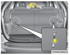
4. Pull on the seatback folding strap, then fold the seat toward the front of the vehicle. When you return the seatback to its upright position, always be sure it has locked into position by pushing on the top of the seatback.
