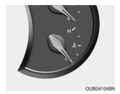
Engine coolant temperature gauge (for Type B cluster)
