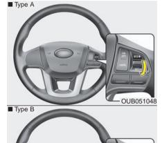
Move the lever (1) down (to SET-), and release it at the desired speed. The SET indicator light in the instrument cluster will illuminate. Release the accelerator at the same time. The desired speed will automatically be maintained.
