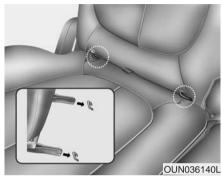
LATCH anchors have been provided in your vehicle. The LATCH anchors are located in the left and right outboard rear seating positions. Their locations are shown in the illustration. There is no LATCH anchor provided for the center rear seating position.
