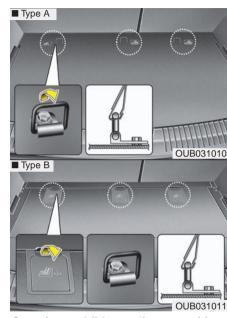
Securing a child restraint seat with tether anchorage system
