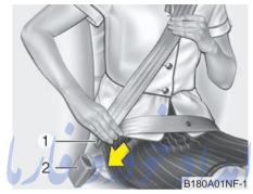
Seat belt - Driver's 3-point system with emergency locking retractor To fasten your seat belt:
