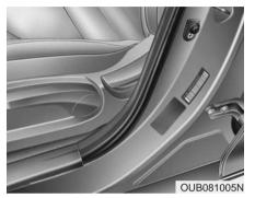
The vehicle certification label attatched on the driver's side center pillar gives the vehicle identification number (VIN).
