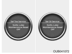
If you would like to reset or inactivate the maintenance system press the RESET button for more than 1 second. The display will change to "Engine Oil Service Message" mode.
