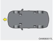
Tie-down hook (for flatbed towing, if equipped)
