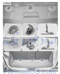
Securing a child restraint seat with "Tether Anchor" system (if equipped)
