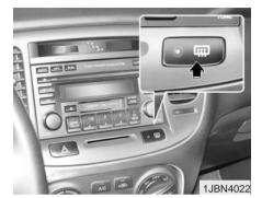
The defroster heats the window to remove frost, fog and thin ice from the interior and exterior of the rear window. while engine is running.
