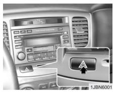
The hazard warning flasher causes the rear tail lights and front turn signal lights to flash on and off, which serves as a warning to other drivers to exercise caution when approaching or passing your vehicle.
