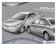
Front air bags may not inflate in side impact collision, because occupants move to the direction of the collision, and thus in side impacts, frontal air bag deployment does not provide occupant protection.
