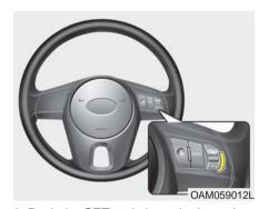
3. Push the SET- switch, and release it at the desired speed. The SET indicator light in the instrument cluster will illuminate. Release the accelerator at the same time. The desired speed will automatically be maintained.
