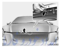
2. Go to the front of the vehicle, raise the hood slightly, pull the secondary latch (1) inside of the hood center and lift (2) the hood.
