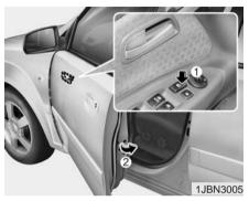
To lock a door without the key, push down on the front portion of the inside door lock switch (1, if equipped) to the "LOCK" position and close the door (2).
