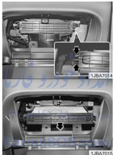
Remove the climate control air filter cover by pressing the clips on both sides of the cover.
