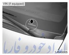
The VIN is also on a plate attached to the top of the dashboard. The number on the plate can easily be seen through the windshield from outside. تلفن شبانه روزي:
