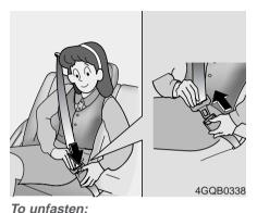
Press the release button on the buckle and allow the belt to slowly retract.
