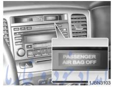
If the passenger in the front passenger's seat is very small, (such as a child), the front PASSENGER AIR BAG OFF indicator may go ON.
