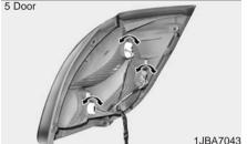
Remove the socket from the assembly by turning the socket counterclockwise until the tabs on the socket align with the slots on the assembly.
