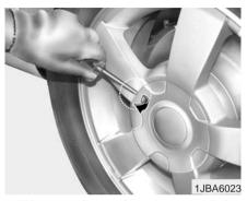
Wrap a piece of cloth around the tip of the screwdriver to avoid scratching.
