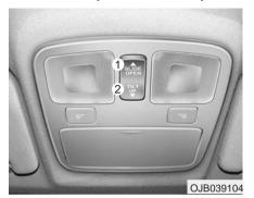
(1) SLIDE OPEN (TILT DOWN) button (2) Tilt UP (slide close) BUTTON
