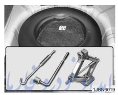
The spare tire, jack, jack handle, front towing hook, wheel lug nut wrench are stored in the luggage compartment. Move the carpeting out of the way to reach this equipment.
