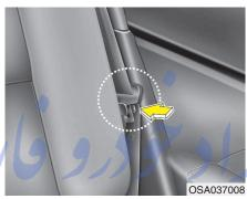
1. Slide the front seat forward and insert the rear safety belt into the belt holder.
