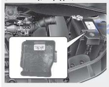
Engine compartment main fuse panel
