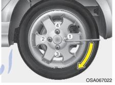
Then position the wrench as shown in the drawing and tighten the wheel nuts. Be sure the socket is seated completely over the nut. Do not stand on the wrench handle or use an extension pipe over the wrench handle. Go around the wheel tightening every other nut until they are all tight. Then double-check each nut for tightness. After changing wheels, have an authorized KIA dealer tighten the wheel nuts to their proper torque as soon as possible.
