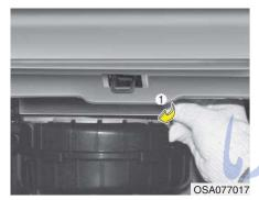
2. Pull out the hooks of the climate control air filter case (1).
