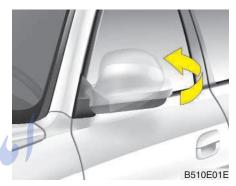
D140202AEN Folding the outside rearview mirror To fold the outside rearview mirror, grasp the housing of the mirror and then fold it toward the rear of the vehicle.
