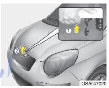
2. Go to the front of the vehicle, raise the hood slightly, pull the secondary latch (1) inside of the hood center and lift the hood (2).
