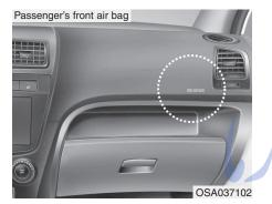
The purpose of the SRS is to provide the vehicle's driver and/or the front passenger with additional protection than that offered by the seat belt system alone in case of a frontal impact of sufficient severity.
