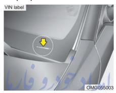
The VIN is also on a plate attached to the top of the dashboard. The number on the plate can easily be seen through the windshield from outside. تلفن شبانه روزي:
