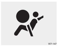
The SRS air bag warning light "\* on the instrument panel will illuminate for about 6 seconds after the ignition switch is turned to the ON position, after which the SRS air bag warning light "\* should go out.
