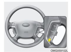
Push the -/SET switch, and release it at the desired speed. The SET indicator light in the instrument cluster will illuminate. Release the accelerator at the same time. The desired speed will automatically be maintained.
