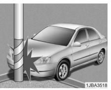
Air bags may not inflate if the vehicle collides with objects such as utility poles or trees, where the point of impact is concentrated to one area and the full force of the impact is not delivered to the sensors C041100AHM
