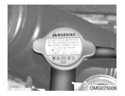
**WARNING** - Radiator cap Do not remove the radiator cap when the engine and radiator are hot. Scalding hot coolant and
