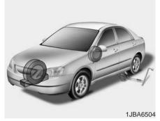
Remove the wheel lug nut wrench, jack, jack handle, and spare tire from the vehicle.
