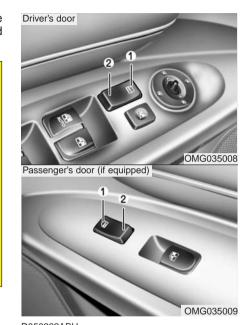
D050202ABH With central door lock switch Operate by depressing the central door lock switch.
